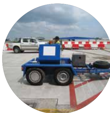
HWD Test at Kuching International Airport
